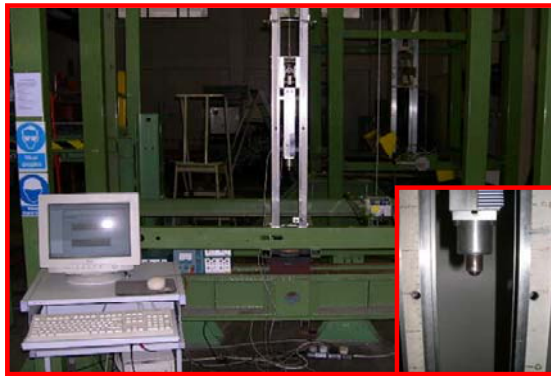
Impact rig and force vs time response of impactor [Donadon et al. 2008].
