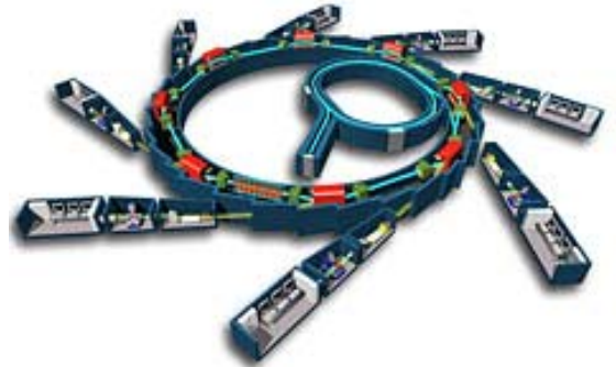
Schematic diagram of a Synchrotron showing accelerator, booster ring, storage ring and beamlines
