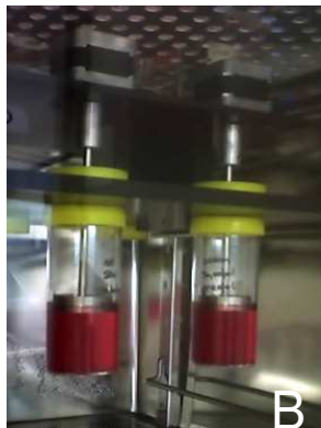
Figure 2 (a). Rotating disc bioreactor rig for mammalian cell culture. (b) Bioreactor set up to contain cell culture fluid under tissue culture conditions inside an incubator .
