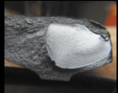
Transverse defects in rail: mass transit
