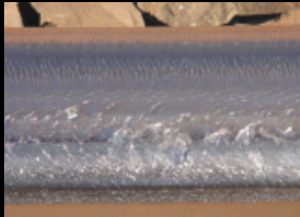
Surface-initiated rolling contact fatigue in rail: heavy haul
