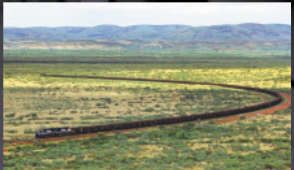
Typical iron ore train carrying approximately 25,000 tonnes of material on a 27 hour turnaround cycle.
