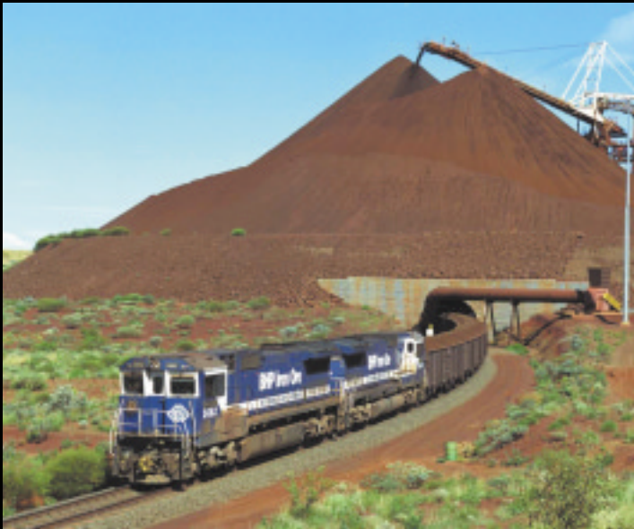
State of the art loading facility at Yandicoogina,, which is consistently producing average axle loads of 37 tonnes.
